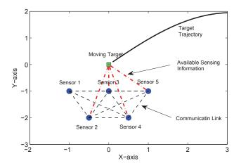
Fig. 1. A group of 5 nodes are deployed in the workspace with the goal of tracking the target. The target is represented by a square, and the sensors are denoted by dots. The sensors form a connected graph, where the dashed link indicates the available communication links. The dashed-dot line connecting the target and the sensor implies whether the sensor is able to measure the target position.
